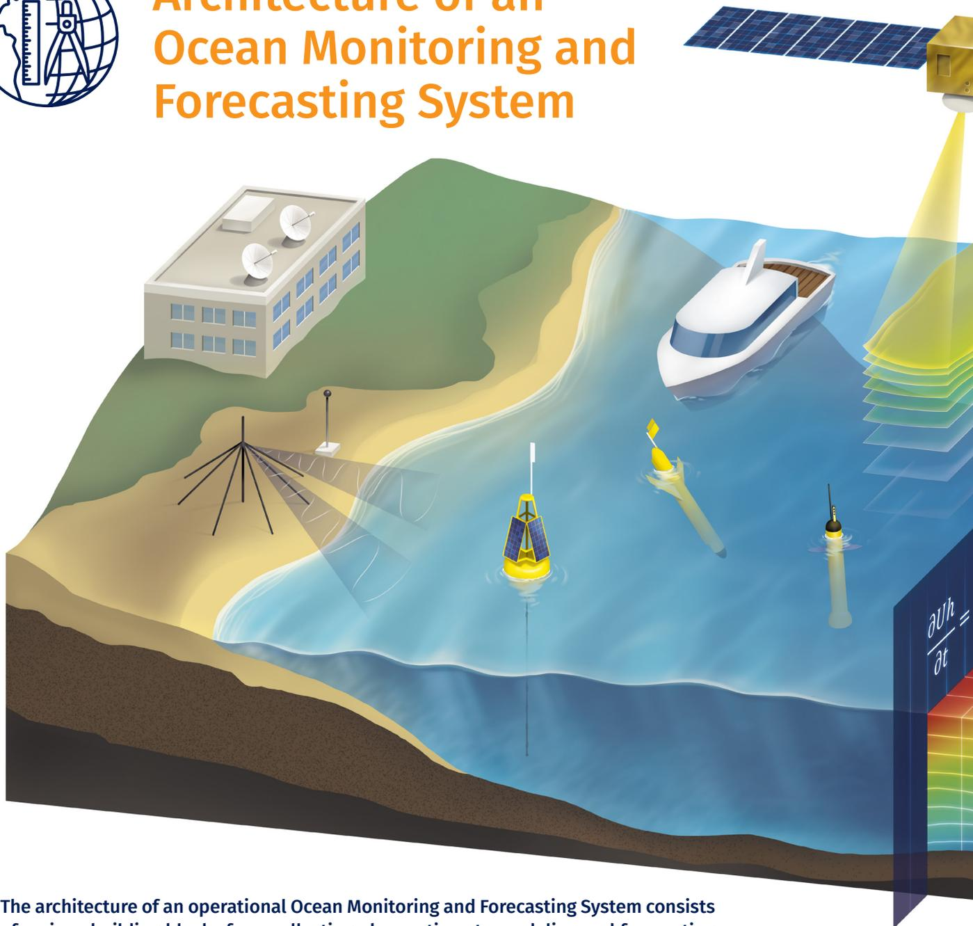
The architecture of an operational Ocean Monitoring and Forecasting System consists of various building blocks from collecting observations to modeling and forecasting the ocean state.
