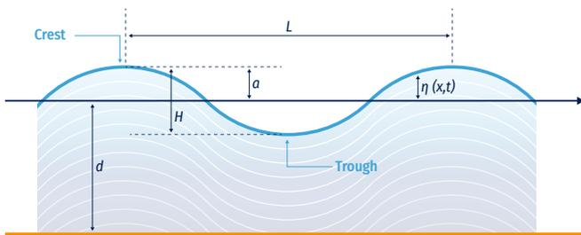
Characteristics of a 2D linear water wave
