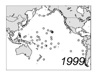
Sea Level Stations – increase from 5 to 74 stations – tsunami detection dropped from 3 hours to 5-30 minutes
