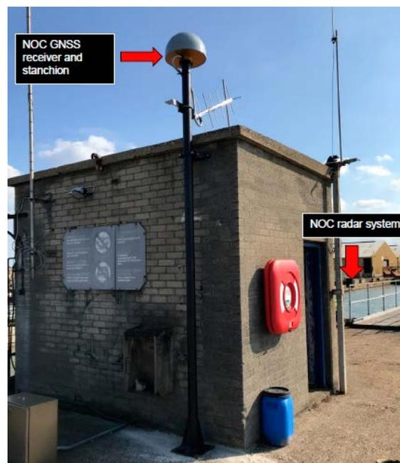
Figure 4. The NOC GNSS system and location relative to the NOC radar system
