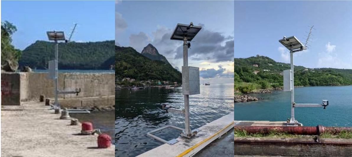
Figure 16. Solar-powered satellite communications-based tide gauges at Dennery (left), Soufriere (middle) and Vieux Fort (right) in St Lucia Solar-powered satellite communications-based tide gauge at Vieux Fort
