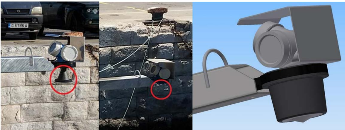
Figure 13: Gibraltar radar gauge showing loss of cone, and design for new cover
