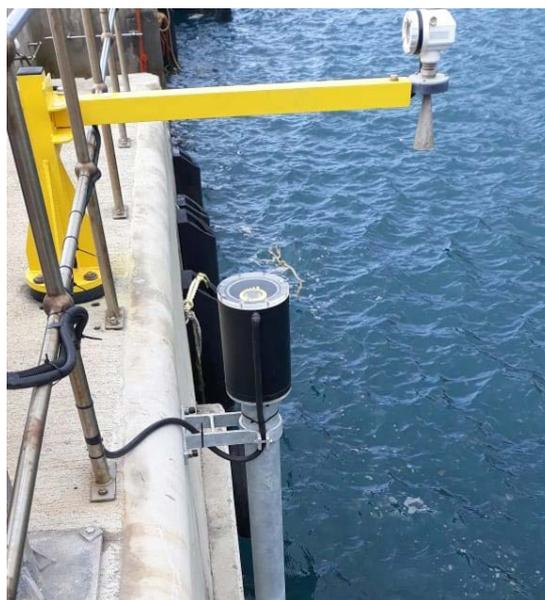
Figure 8: St Helena new stilling well, alongside open water radar gauge
