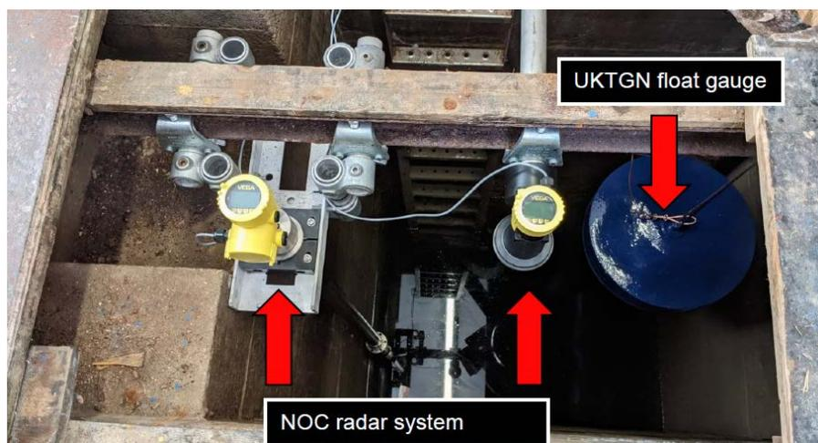
Figure 2: Observatory stilling well containing the NOC radar system and the UKCFF float gauge
