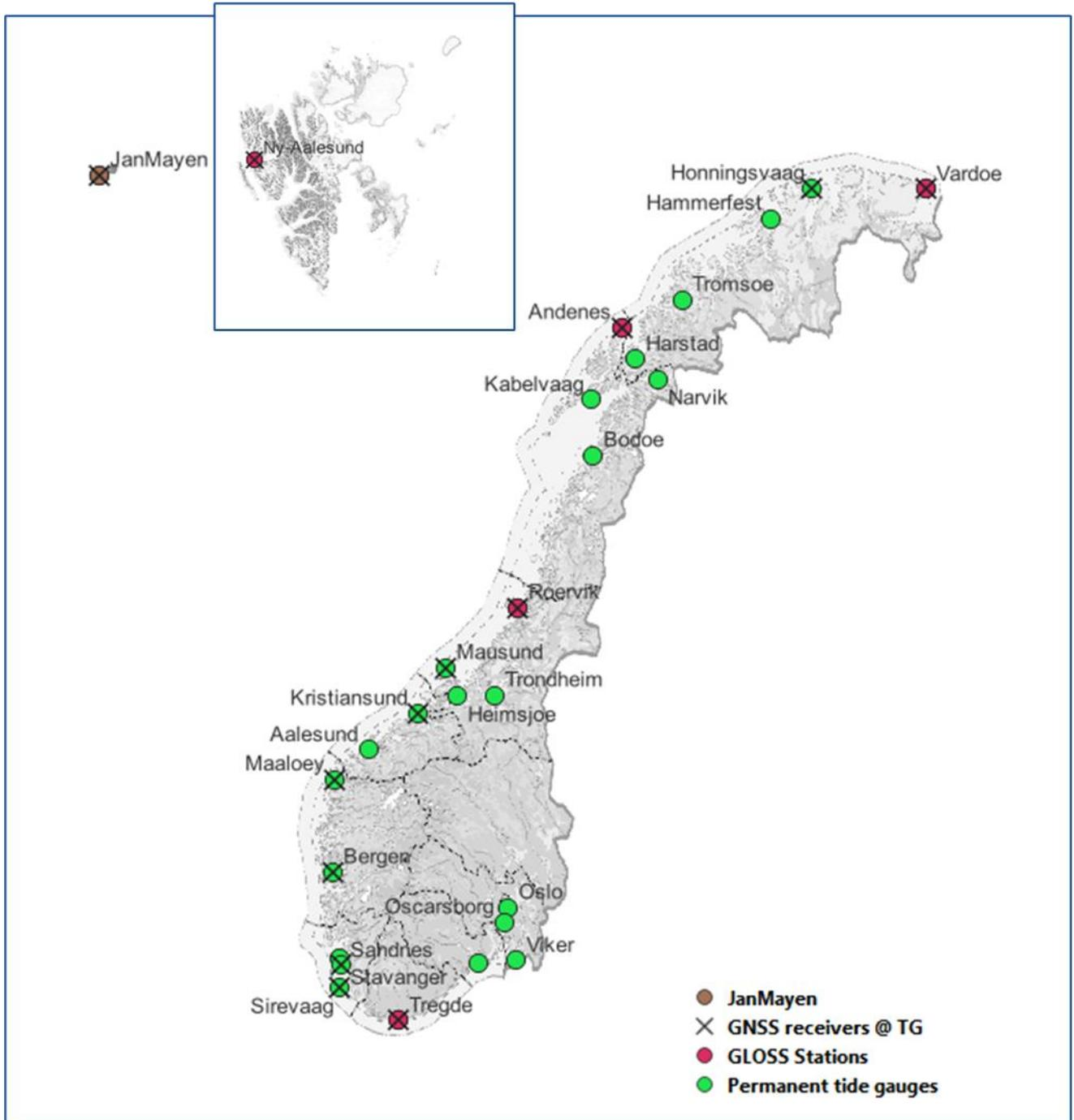
Figure 1: Overview of Norwegian tide gauges, GLOSS stations and GNSS receivers co-located with tide gauges
