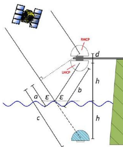
**Figure 11.** An upward- and downward looking GNSS-reflectometer.
