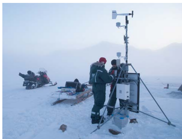
Figure 9. Field work and installation of new sensors at the permafrost monitoring station at Janssonhaugen (78°N) on Svalbard on a cold day in mid-February. Photo: Ketil Isaksen)
