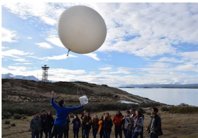
Figure 1. Ozonesonde observation at Pohang (GAW ID: POH). Ozonesondes measure ozone and meteorological variables at different altitudes as the sonde ascends, until the balloon bursts. (Source: KMA)
